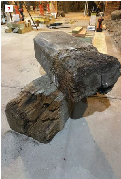
The bottom ends of the columns were rotted below the slab but perfectly sound about 2 feet above the floor (7). Using a rotary hammer, the author chipped out the old slab around the column for new footing pads (8).
