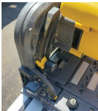
The depth and bevel controls are readable and accurate, with bevel locks at both front and back (left). With the author’s kit he can break down sheets, prefinished doors, and panels (right).
