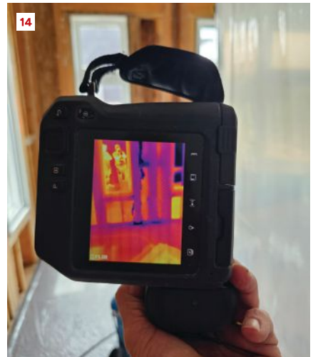
Deterioration of the OSB sheathing (12) was discovered where brick tie fasteners (circled in red) penetrated the sheathing, instead of being driven into framing (13). An infrared image (14) highlights moist areas in darker colors where water has run down the wall cavities and started to deteriorate the bottom wall plates.
