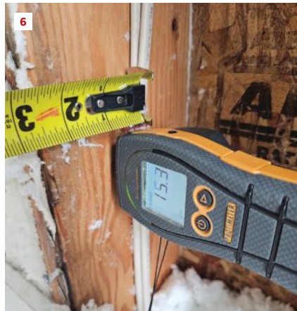
Taking readings across the stud, the author recorded the highest moisture levels along the inside edge (5), with the levels dropping off as he took measurements toward the exterior (6, 7).
