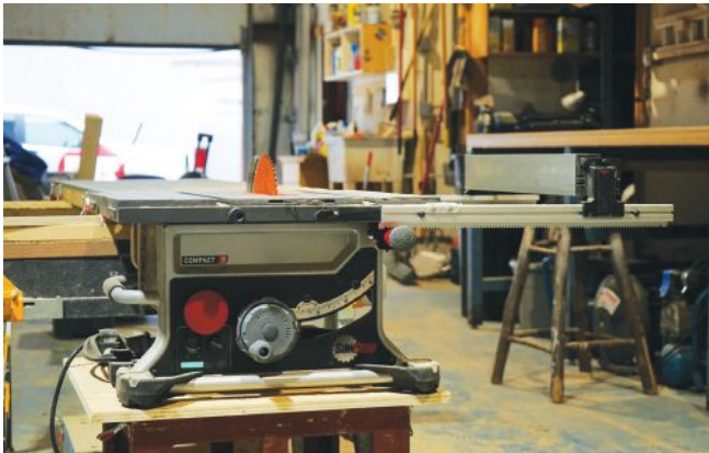
The SawStop CTS provides 24 ½ inches of supported rip capacity with a sturdy base—the saw weighs 68 pounds.
