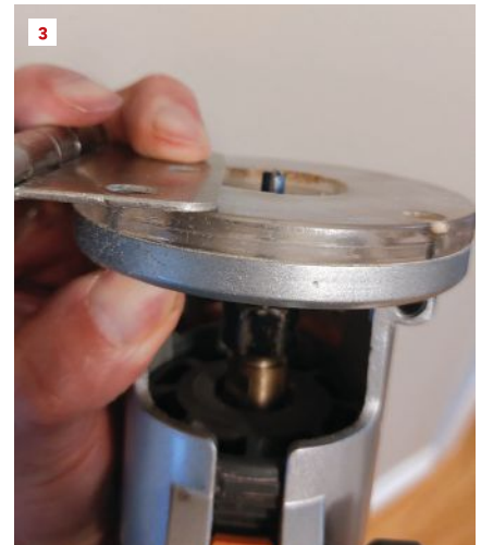
Start small then build up as you need. A few bits will do most jobs (2). Setting the depth for the hinges? Just use the hinge as a guide (3). Be sure to do a test run before touching finish material.
