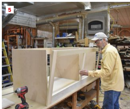
The author pocket-screws the face frames (1) and rabbets the panels for the carcasses (2). Next, he glues, screws, and staples the boxes and back panels (3, 4). Then, he mounts the frames (5) and builds the drawers (6).
