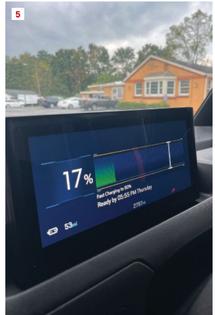
Charging at a DC fast charger is not much different from filling up at a gas station, except it takes longer. To maintain battery health, GM sets the maximum charge to 80%; it also recommends charging the battery when its capacity decreases to about 20%.
