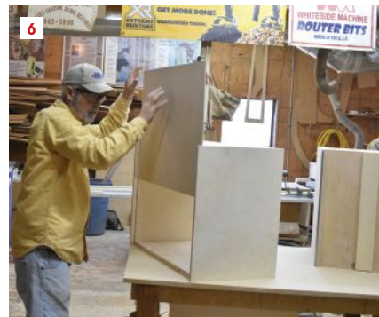
The author pocket-screws the face frames (1) and rabbets the panels for the carcasses (2). Next, he glues, screws, and staples the boxes and back panels (3, 4). Then, he mounts the frames (5) and builds the drawers (6).
