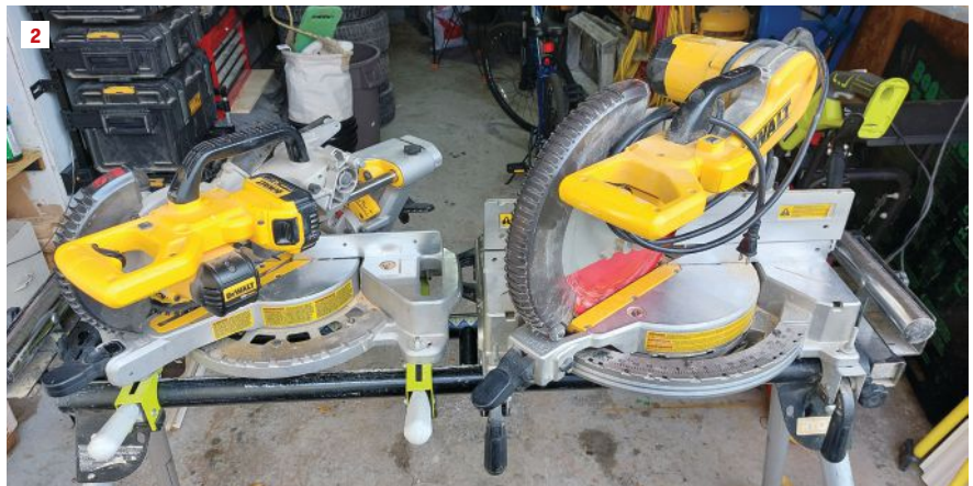
The DeWalt DCS361M1, with its open side grips and a top handle, is easy to move around a jobsite (1). Note the difference between the 7 ¼- and 12-inch saws (2). Not every job needs the biggest tool.
