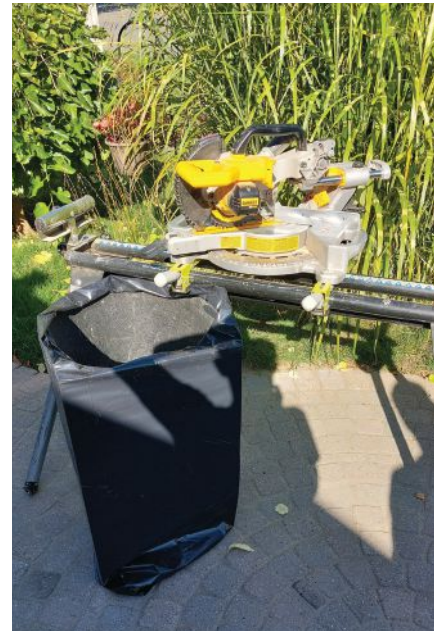
This bin, a yard-bag insert inside a garbage bag, stores flat and takes up little space (above).
