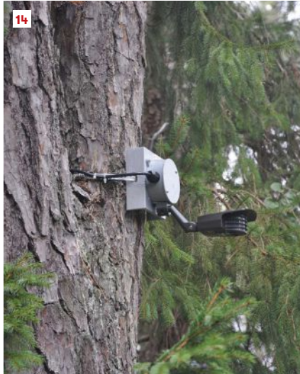
Light and motion sensor. The author mounted the brackets holding the LED light fixture (13) and motion sensor (14) on the tree with stainless-steel straps. The motion sensor is positioned lower on the trunk, which stands about 12 feet from the old utility pole on which the control box is mounted.
