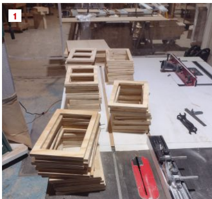
By making all the boxes the same size, the author saved on materials and construction time. This uniformity means an accessory built for one will fit all. The boxes can also be stacked to create level worktops (1, 2). The author can easily adjust the drawer dividers as his needs change (3).
