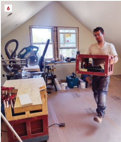
The author says the boxes are easy to carry and provide a sturdy platform to stand on (6, 7). With the system set up as a miter station, the hold-down clamps keep everything secure, including tall and short drawers, open storage, and dust collection, all in a single mobile unit (8).
