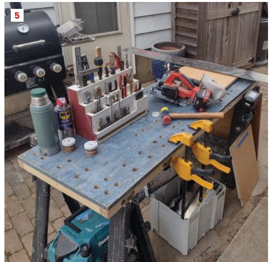
The holdowns on the boxes enable clamping them together as a unit for secure stacking in the author’s van (4). The worktops provide a flat work surface for many tasks. Note the drilled holes for clamps as well as the clips on the edges for hanging tools within easy reach (5).
