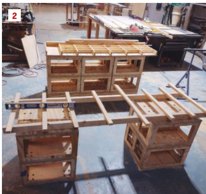
By making all the boxes the same size, the author saved on materials and construction time. This uniformity means an accessory built for one will fit all. The boxes can also be stacked to create level worktops (1, 2). The author can easily adjust the drawer dividers as his needs change (3).
