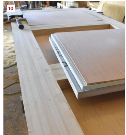
These are some of the options that could be used to fit the door frame (from left to right in the photo) (6): Domino XL, dowels, and regular Domino. After touch-up sanding at the joints (7), the author spreads glue for the first skin of the door (8). With the first side glued and clamped (9), he fills the door voids with rigid foam and plywood (10).
