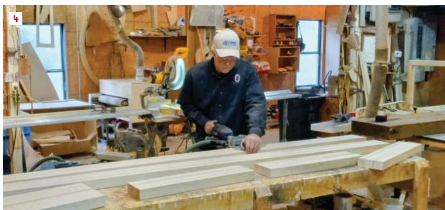
Planing the lumber for the stiles before glue-up ensures clean and flat surfaces (1, 2). The author built a sled to plane the larger glue-ups to final thickness. Shims prevent the material from rocking (3). For alignment and strength, Domino XL tenons are used for the attachment of the door rails and stiles (4, 5).
