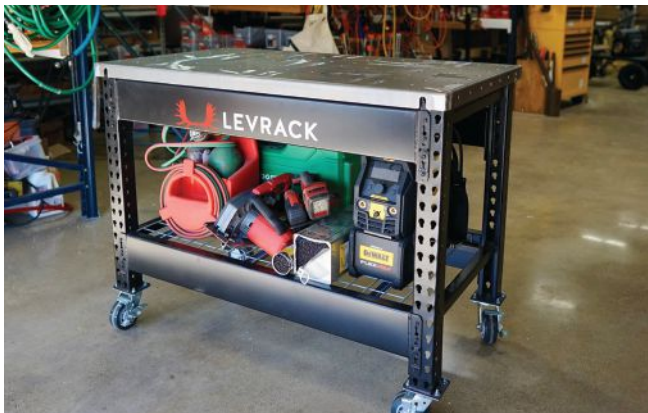
The Levrack 4-foot (actual length is 55 inches) workstation has a robust work surface with holes for mounting tools as well as a storage shelf underneath. The table pictured is 30 inches wide; it can be ordered with a solid or perforated top by special request.
