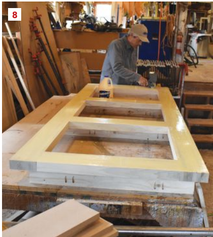
These are some of the options that could be used to fit the door frame (from left to right in the photo) (6): Domino XL, dowels, and regular Domino. After touch-up sanding at the joints (7), the author spreads glue for the first skin of the door (8). With the first side glued and clamped (9), he fills the door voids with rigid foam and plywood (10).
