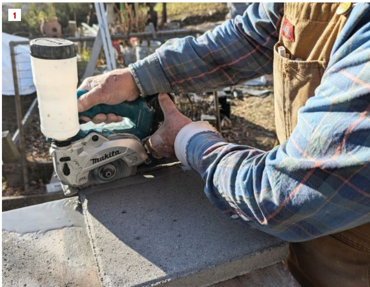
A 12-ounce bottle provides adjustable water flow to keep down dust (1). For constant water feed, a hose attachment can be used instead. Depth of cut on the compact, 6.6-pound Makita XCC01Z can be set with its adjustable baseplate (2).
