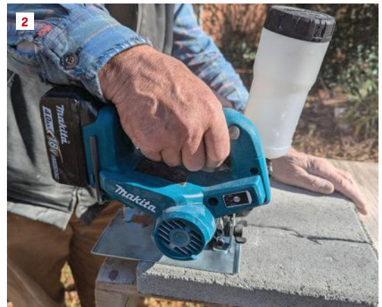
A 12-ounce bottle provides adjustable water flow to keep down dust (1). For constant water feed, a hose attachment can be used instead. Depth of cut on the compact, 6.6-pound Makita XCC01Z can be set with its adjustable baseplate (2).
