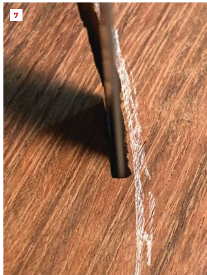
Here, the author is top scribing. The part marked with a “4” is the set edge and the one marked with a “7” is the mating edge (6). The author makes a side-cut in the Brazilian cherry that will have the bottom part of the ball set into it (7).
