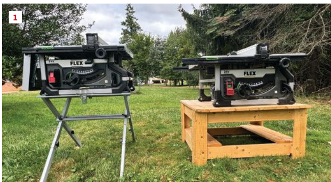
The Flex cordless table saw is available in 8 1/4-inch (on stand, at left in photo) and 10-inch (on table, at right in photo) models (1). The stand can be configured for either model. The author operates the fold-out support of the 8 1/4-inch saw (2).
