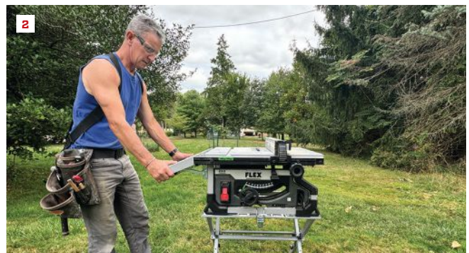
The Flex cordless table saw is available in 8 1/4-inch (on stand, at left in photo) and 10-inch (on table, at right in photo) models (1). The stand can be configured for either model. The author operates the fold-out support of the 8 1/4-inch saw (2).
