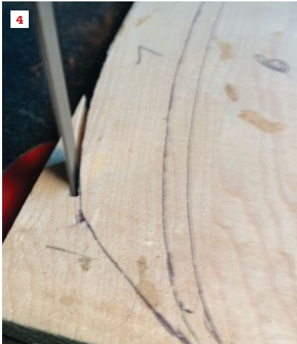
Here is an example of a through-cut in a section of maple. A slight back bevel allows for easier fine-tuning later (4). A darkened finger tip run along the edge of the wood on the paper creates a crease and an easy-to-see line. Cutting along this line will make a template (5).
