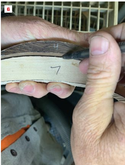
Here, the author is top scribing. The part marked with a “4” is the set edge and the one marked with a “7” is the mating edge (6). The author makes a side-cut in the Brazilian cherry that will have the bottom part of the ball set into it (7).
