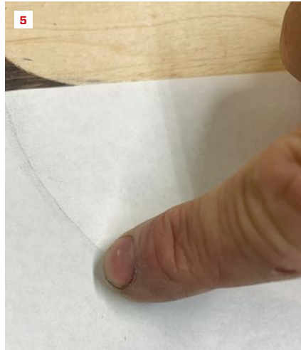
Here is an example of a through-cut in a section of maple. A slight back bevel allows for easier fine-tuning later (4). A darkened finger tip run along the edge of the wood on the paper creates a crease and an easy-to-see line. Cutting along this line will make a template (5).
