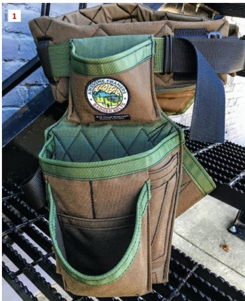
The pouches on Badger’s toolbelt stay open and are large for easy access but not so deep that items become buried (1). The padded belt helps keep the wearer comfortable while working (2).
