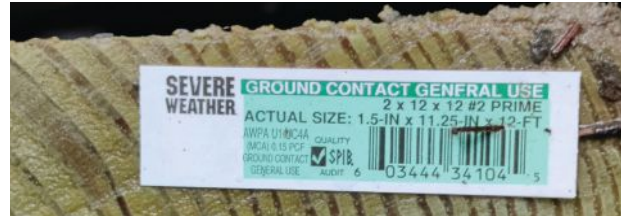
Preservative treatment lumber tag on one end gives the size of the 2x12, along with the AWP UC4A level that indicates it is suitable for “Ground Contact.”
