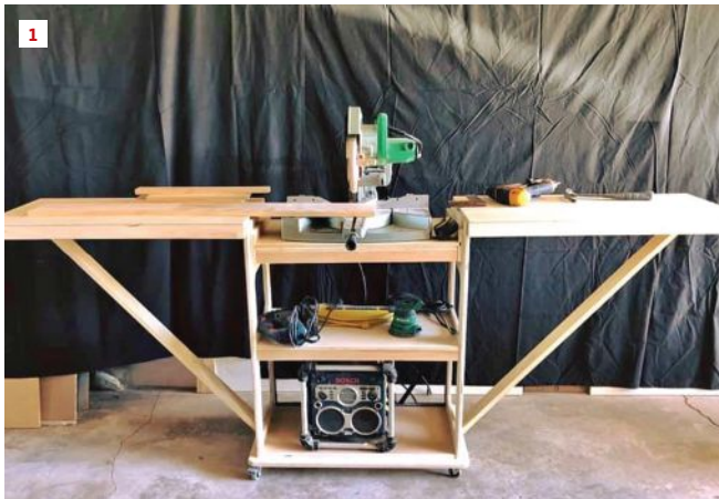
The author’s original miter saw stand (1) worked well but had limited other uses and was bulky. He replaced it with a plywood sawhorse system that can be broken down into flat pieces for transport (2).
