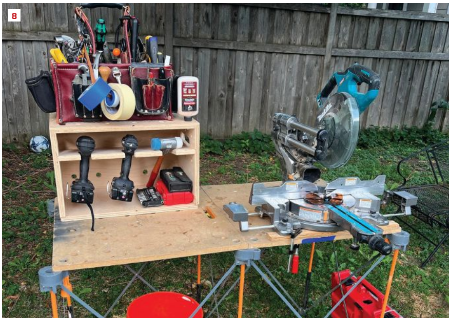
Lightweight workbench. For smaller jobs, the author sets up a simple workstation built on a Centipede CK6S stand (8), which is easy to set up and break down and light to transport. Often for these smaller jobs, he brings what he needs from the truck in an Occidental carpenter case (9). He often carries a portable cordless case (10), similar to his larger rolling case. It is sized to fit on the Milwaukee Packout system, and doubles as a step stool and task oriented workstand (11).
