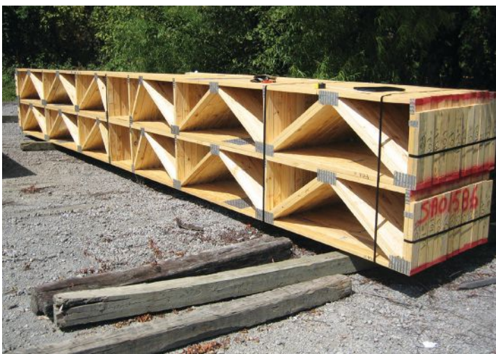
Figure 1. In a typical floor system framed with truss joists, a nonstructural ribbon board is attached to the top of the floor trusses. This 2x4 ribbon board is not intended for a deck ledger attachment.
