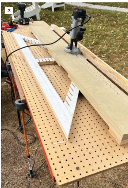
The author builds a jig that bridges across the top of a frame for a gable-end vent. Shelf pins in the jig register in the holes on the pegboard work surface (1). The top of the jig is made from two layers of beveled siding that position a plunge router at an angle (2). By running the router along a slot in the jig, he cuts angled mortises across all three members of the frame (3).
