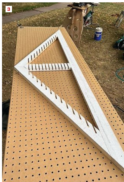
The author builds a jig that bridges across the top of a frame for a gable-end vent. Shelf pins in the jig register in the holes on the pegboard work surface (1). The top of the jig is made from two layers of beveled siding that position a plunge router at an angle (2). By running the router along a slot in the jig, he cuts angled mortises across all three members of the frame (3).
