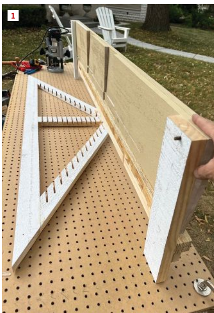
The author builds a jig that bridges across the top of a frame for a gable-end vent. Shelf pins in the jig register in the holes on the pegboard work surface (1). The top of the jig is made from two layers of beveled siding that position a plunge router at an angle (2). By running the router along a slot in the jig, he cuts angled mortises across all three members of the frame (3).
