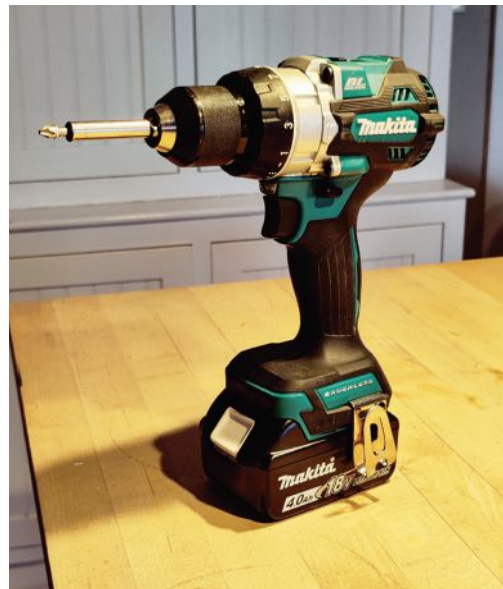
The Makita XPH14 18V LXT hammer drill/driver has a powerful, high-torque motor.
