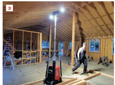
The Milwaukee MX Fuel Rocket Tower light extends to 10 feet (1) and puts out as much as 27,000 lumens, enough to fully illuminate the side of a house or a cavernous workspace (2, 3).
