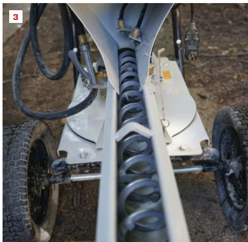
The mixing is done by an auger running the length of the narrow, horizontal chute (3).
