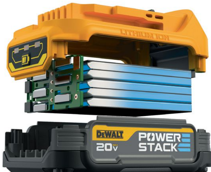
In this cut-away image of a DeWalt 20-volt lithium-ion battery, the five rectangular silver objects are 4-volt pouch cells that are wired together in series to provide 20 volts of power. The green board is the module that electronically controls the battery.
