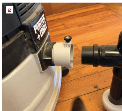
The parabolic cyclone that forms the top section of the Mullet M5 Cyclone Dust Collector scrubs dust particles out of the air before they fill up the vacuum cleaner bag or clog up the filters (1). A simple thumbscrew connects and disconnects the Mullet from the vac with ease (2). Every time the 5-gallon-capacity dump bin fills up, a dust bag lives to fight another day (3).
