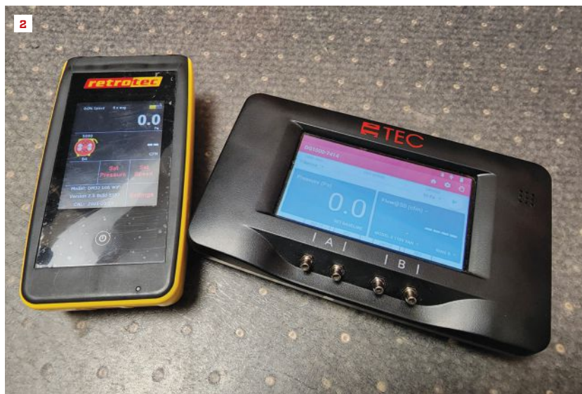
Two digital manometers (2): Retrotec DM32 (above, at left) and The Energy Conservatory DG-1000 (above, at right). Before the creation of the modern digital gauges, analog Magnehelic pressure gauges were used to perform blower door tests. This set (3) was part of an early (around 1990) Minneapolis Blower Door system.
