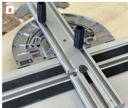
Fitting a Festool track-saw guide rail with the FS-WA angle stop and FS-WA-VL guide extension gives the saw the ability to make repeatable miter cuts at angles up to 60 degrees (1). The angle stop includes a pair of black positioning bolts that can be locked into the stop's T-track slots (2). The FS/2-Set includes the stop and other accessories and a Systainer (3).
