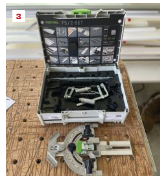
Fitting a Festool track-saw guide rail with the FS-WA angle stop and FS-WA-VL guide extension gives the saw the ability to make repeatable miter cuts at angles up to 60 degrees (1). The angle stop includes a pair of black positioning bolts that can be locked into the stop's T-track slots (2). The FS/2-Set includes the stop and other accessories and a Systainer (3).
