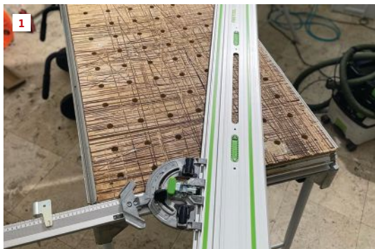
Fitting a Festool track-saw guide rail with the FS-WA angle stop and FS-WA-VL guide extension gives the saw the ability to make repeatable miter cuts at angles up to 60 degrees (1). The angle stop includes a pair of black positioning bolts that can be locked into the stop's T-track slots (2). The FS/2-Set includes the stop and other accessories and a Systainer (3).
