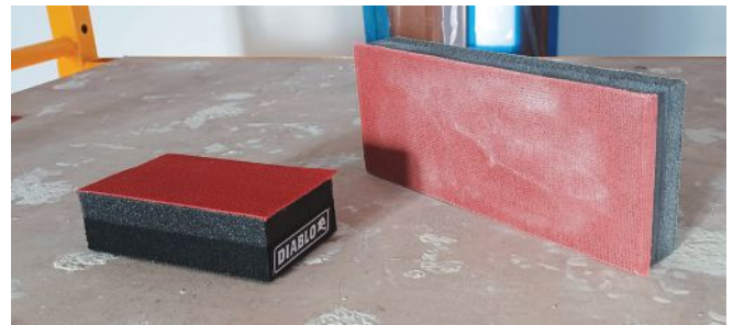
One sheet of 220-grit SandNet (on long foam block at right) sanded more than 1,110 square feet of skim-coated plaster.
