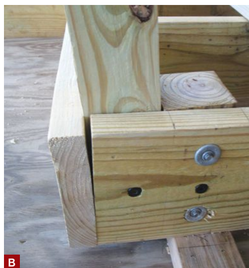
Figure 1. The author used a hand cable winch fitted with a 1,500-lb. digital crane scale to informally test the strength of different guard-post-to-frame connections made with structural screws and blocking (A). His goal was to see how these connections would fare under the 500-lb. test load requirement of ASTM D7032, the standard that wood-plastic composite (WPC) guardrail systems have to meet to comply with code (B).
