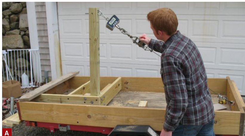
Figure 1. The author used a hand cable winch fitted with a 1,500-lb. digital crane scale to informally test the strength of different guard-post-to-frame connections made with structural screws and blocking (A). His goal was to see how these connections would fare under the 500-lb. test load requirement of ASTM D7032, the standard that wood-plastic composite (WPC) guardrail systems have to meet to comply with code (B).
