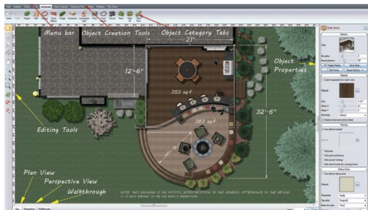
Figure 1. Plan view mode in Realtime Landscaping Architect (indicated in the bottom left corner of the screen) includes all the information shown in the screen shot above, such as the menu bar, object category tabs, and object creation tools. On the left side of the screen are icons for editing tools, view tools, and grid/snap on and off. On the right-hand side of the screen, all the information about a highlighted object is shown. This information will not show up in the 3D renderings in either Perspective or Walkthrough views.
