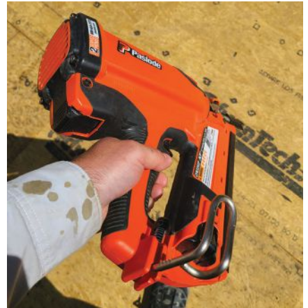
The Paslode XP nailer has a big rafter hook that rotates so that the nailer can also be hung from a tool belt.
