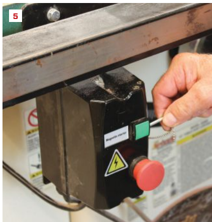
A custom zero-clearance throat plate adds critical full support under small and narrow workpieces, which might otherwise jam dangerously in the gap. Here, a 1/4-inch dado stack is raised through its dedicated plate (4). A switch key locks out unwanted saw activation when the author is setting up or changing blades (5). A digital angle indicator ensures the accuracy of bevel cuts (6).
