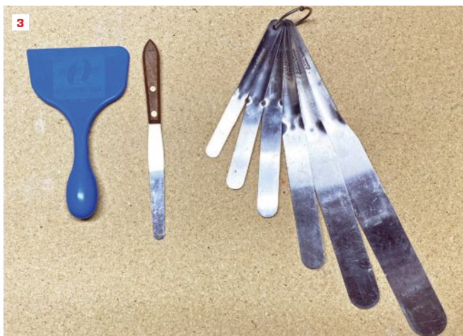
Tooling a caulk joint ensures it beds well against backer rod (Butt Joint illustration, top right) or against a substrate (Fillet Joint, bottom right). Almost anything with a smooth, curved edge will work. The author likes the blue plastic flashing tool shown in the photo (3). Also shown (center and right in photo) are a single spatula and spatula set, from Albion.
