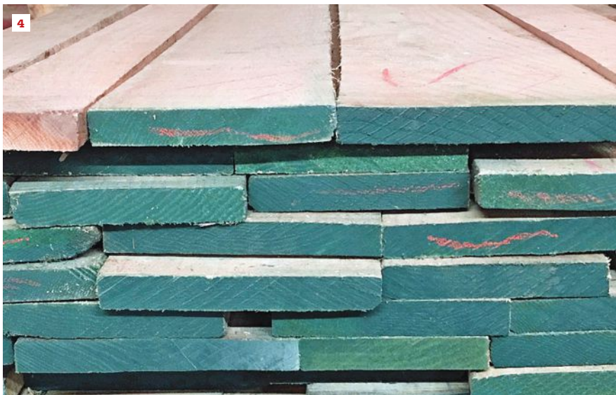
The majority of lumber at a hardwood dealer is rough sawn. Here are three rough, live-sawn logs (3). When available, having them stacked like this makes it easy to match grain. Dealers may also bundle S2S material (4), with two sides surfaced to an even thickness but both edges left rough, so the boards will be of varying width.
