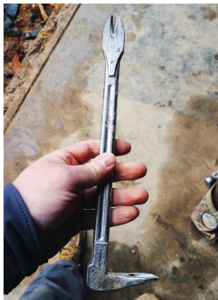
The Dalluge Da Bar is a tough nail puller with flat claws that can slip easily under trim without damaging it.
