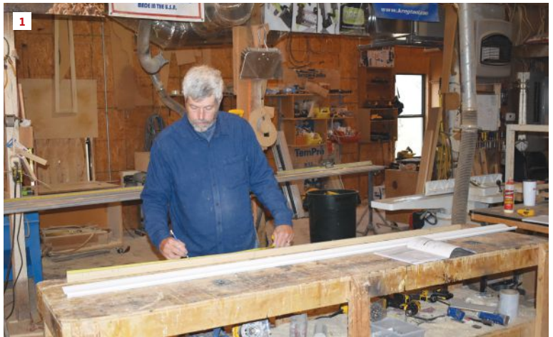
The author marks the height, width, and noncombustible clearance dimensions of the fireplace on a story pole, then lays out the mantel design in full scale (1). Only three different stock molding profiles were used to build the mantel in this story.
