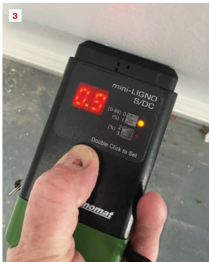
The scale on the author’s Mini-Ligno (3) is set for drywall, for which 1% moisture content (MC) is the trigger point; a higher value would indicate an elevated moisture condition. The author finds that the readings from this relatively inexpensive pin meter from Calculated Industries (4) compare favorably to the ones from his other meters. The Delmhorst ProScan (5) can read wood moisture content to a depth of \frac{3}{4} inch without marring finished surfaces.
