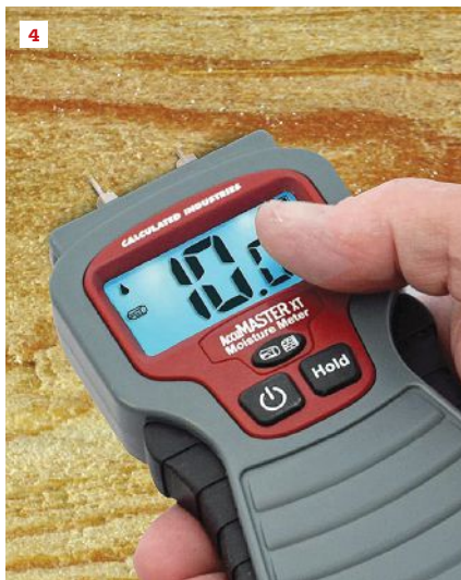
The scale on the author’s Mini-Ligno (3) is set for drywall, for which 1% moisture content (MC) is the trigger point; a higher value would indicate an elevated moisture condition. The author finds that the readings from this relatively inexpensive pin meter from Calculated Industries (4) compare favorably to the ones from his other meters. The Delmhorst ProScan (5) can read wood moisture content to a depth of \frac{3}{4} inch without marring finished surfaces.
