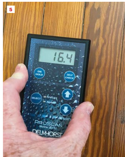
The scale on the author’s Mini-Ligno (3) is set for drywall, for which 1% moisture content (MC) is the trigger point; a higher value would indicate an elevated moisture condition. The author finds that the readings from this relatively inexpensive pin meter from Calculated Industries (4) compare favorably to the ones from his other meters. The Delmhorst ProScan (5) can read wood moisture content to a depth of \frac{3}{4} inch without marring finished surfaces.
