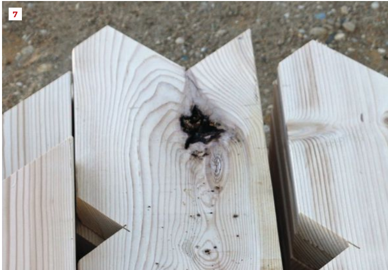
Bark pockets often occur when bark gets trapped by the tree's growth at the crotch of a tree, evident here (7) by the grain pattern of the center board. Interlocked grain can be identified by bands of alternating grain (8), as in this purpleheart board at right, which is shown next to a pine board for comparison.
