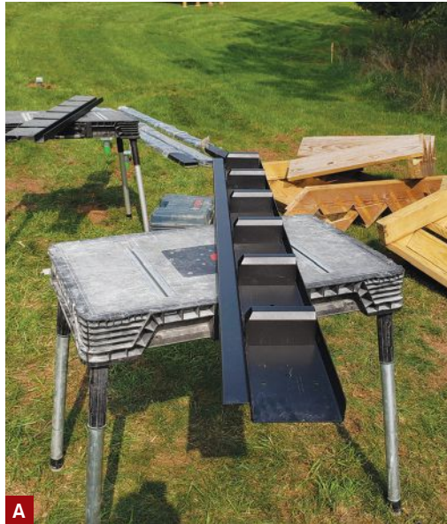
Figure 1. In the Evolution system, ledger brackets are screwed to the S-ledge, or fit into punched openings in the S-ledge without requiring additional fasteners (A). In comparison, an LGS ledger track has bent tabs for fastening the joists to the ledger (B) and requires five or more fasteners per joist-to-ledger connection. Evolution joists just slip over the brackets, and are held in place with a pair of screws per bracket (C).
