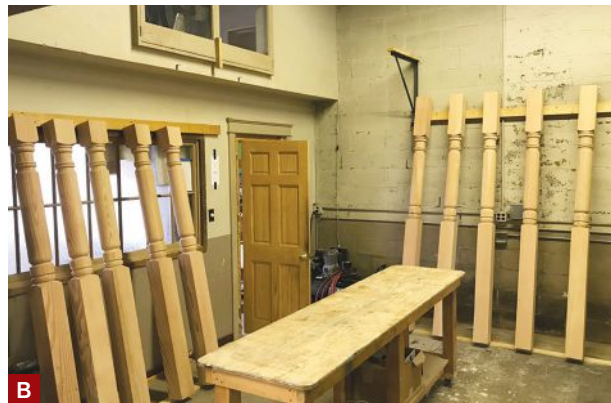
Figure 3. Per local code, the pressure-treated framing was covered with painted wood trim to help maintain the original look of the house; blocking between the framing and wood trim allows moisture to escape from the assembly (A). A local craftsman turned the custom 6x6 Douglas fir posts (B), which the author primed and painted prior to installation (C).
