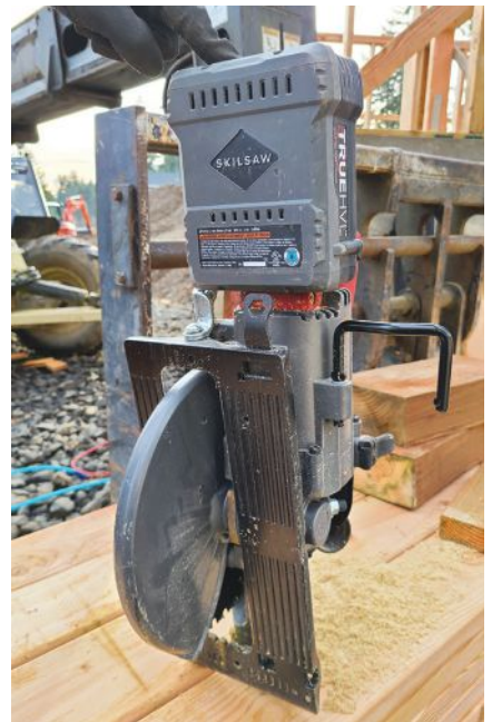
The blade-left saw, which has an electric brake and a built-in dust port, can be tilted to make bevel cuts of up to 51 degrees (left). It also features a rafter hook, which the author found works fine on rafters, but not so much on sawhorses (right).
