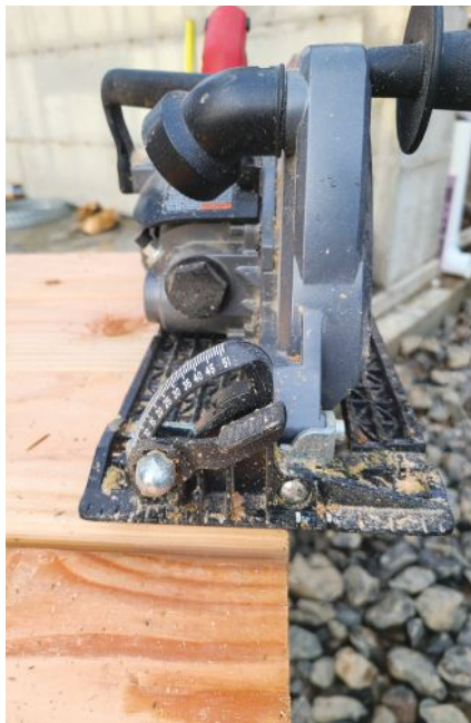
The blade-left saw, which has an electric brake and a built-in dust port, can be tilted to make bevel cuts of up to 51 degrees (left). It also features a rafter hook, which the author found works fine on rafters, but not so much on sawhorses (right).
