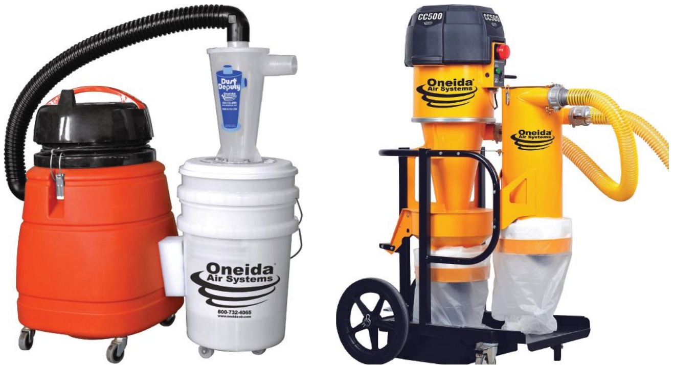
Cyclonic dust extractors can suck up large volumes of dust without clogging filters. Large stationary units are common in woodworking shops, but there are several portable types available now, as well. At left is an “add-on” version, which requires you to use your own vacuum; at right is an all-in-one unit.
