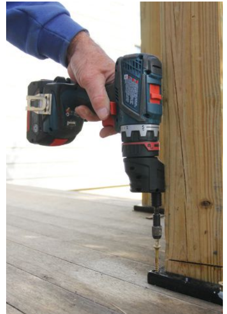
Bosch's Flexiclick drill/driver comes with three attachments, including an offset-angle attachment for driving fasteners close to an adjacent surface (left, right). Its integral 1/4-inch hex bit allows it to be operated without any attachment (center).
