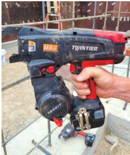
The Max TwinTier is about twice as fast as the Makita and has a larger jaw, allowing it to tie up to #7 x #7 rebar.
