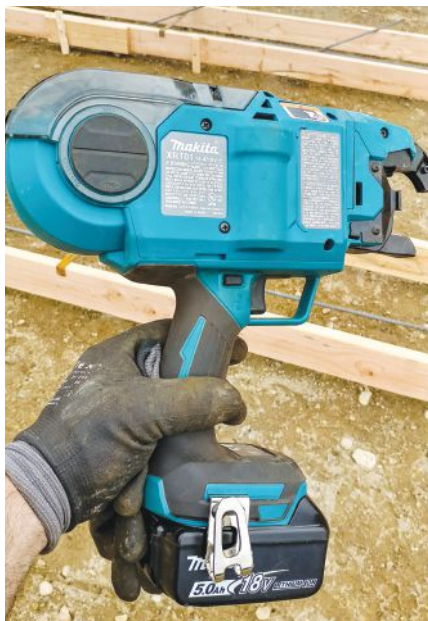
The Makita LXT rebar tier uses #3 wire and has a plastic cover to keep moisture and dirt out of the tying mechanism.
