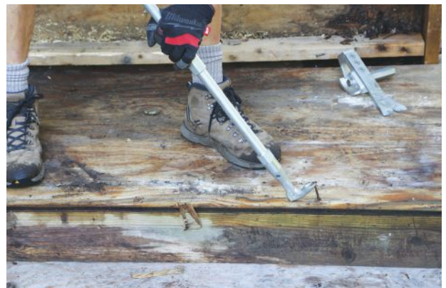
The standard, 25-inch-long steel handle (at top in photo, above left) can be fitted with a ball grip and shorter extensions for more comfort and better leverage. Specialty heads like this nail puller (above right) screw directly onto the handle.
