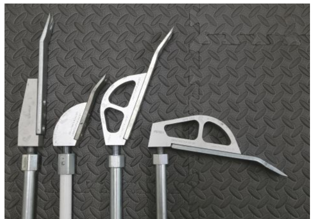
The fulcrums, which determine the angle of attack, can be fitted with different blades (above, from left to right): scraping; mini; standard; deck and drywall.
