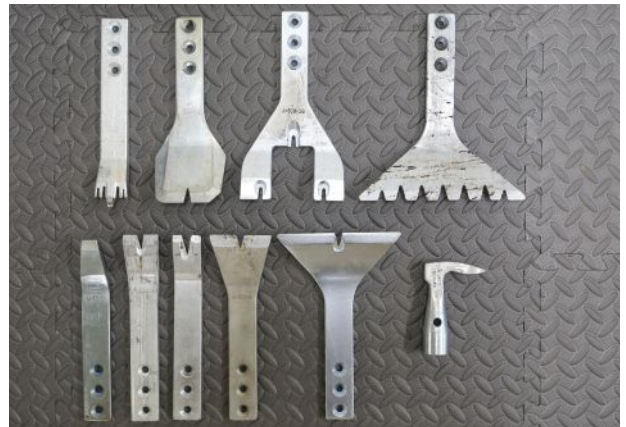
The salvage blade is useful for stripping siding (above left). Other blades include (above right, top row) finish nails; salvage; decking; 8-inch; and (bottom row) \frac{3}{4} -inch; 1\frac{3}{4} -inch; spike puller; 3-inch; 6-inch; and buried nail-head puller.
