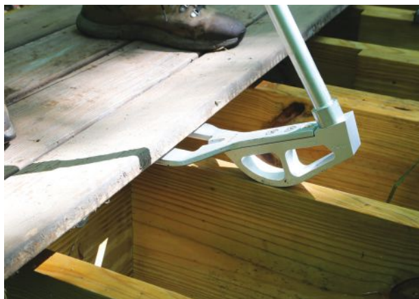
Here, the Artillery Tools kit has been fitted with the deck and drywall fulcrum, the U-shaped removal blade, and both a 12-inch handle extension and a 25-inch handle.
