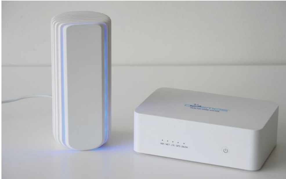
The Foobot pollution sensor (at far left) communicates through the Cosmos control center (at left).
