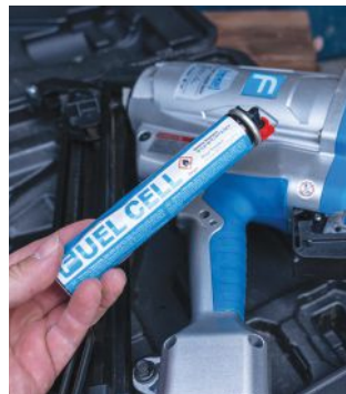
The gun is powered by a fuel cell (left), which slides into the back of the tool (right).
