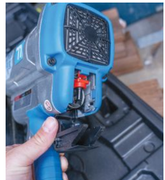
The gun is powered by a fuel cell (left), which slides into the back of the tool (right).
