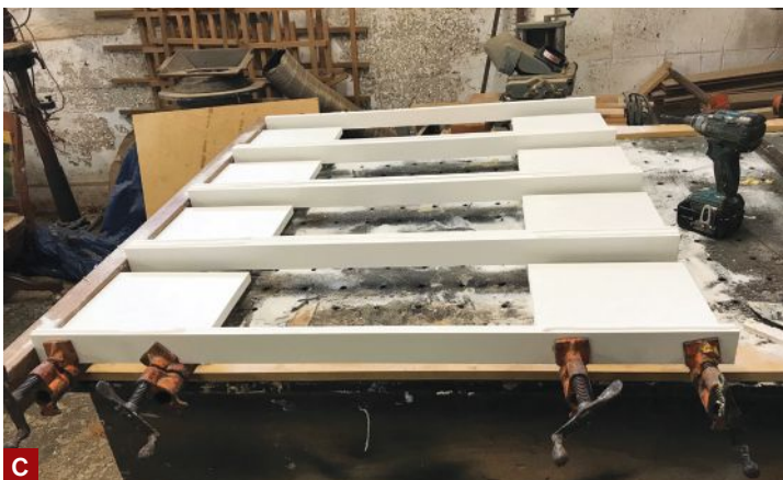
Figure 1. After cutting the stiles and rails to size from \frac{3}{4} -inch-thick PVC stock and setting up his gluing station (A), the author used fast-cure PVC cement to glue up the frames one at a time (B). Switching to a slow-cure adhesive allowed him to glue up several frames at once (C), but the frames needed to remain clamped for an hour.
