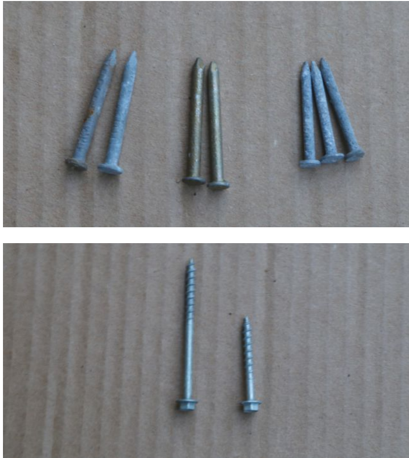
Figure 4. Be sure to match the nail diameter and length to the joist-hanger manufacturer's requirements (top). If you are using connector screws (bottom), they must be the same brand as the hardware and approved for use with the specific hardware you're installing.
