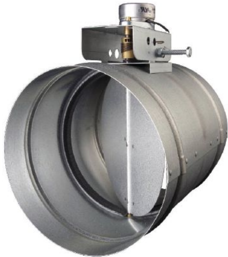
Broan's makeup air damper opens or closes in response to the control on the range hood fan, allowing passive entry of makeup air for the exhaust fan.
