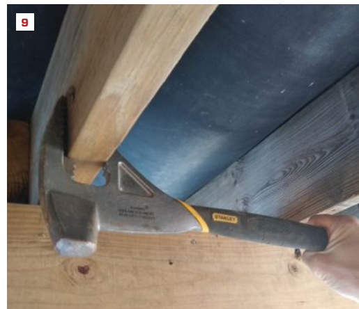
The jaws of the Mayhew Tweaker (8) and the Stanley FuBar (9) are designed to grip the edge of 2-by framing so that twisted joists can be easily leveraged into position with one hand.
