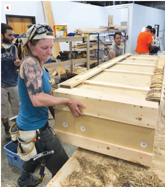
Panel assembly takes place on tables at a convenient working height (4). This panel has Gutex fiberboard insulation, rainscreen strapping, and corner protection applied. Above, a closeup of the panel in cross section (5).
