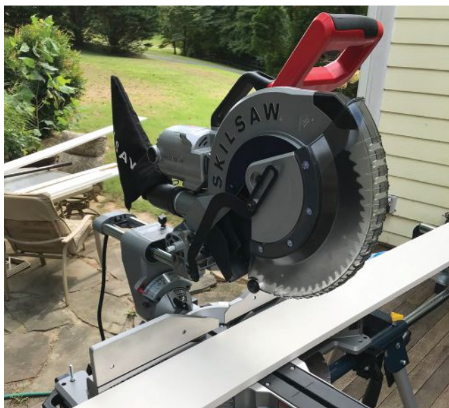
Skilsaw's powerful SPT88 wormdrive dual-bevel 12-inch SCMS has a big footprint, yet weighs in at only 51 pounds.
