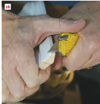
A coping foot mounts on a jigsaw in place of the footplate. The top three photos (12-14) show a typical sequence. For a mitered look, cut the angled sliver (15) and make a relief cut in the mating piece (16) so the two sides fit together (17).
