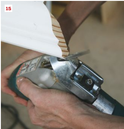
A coping foot mounts on a jigsaw in place of the footplate. The top three photos (12-14) show a typical sequence. For a mitered look, cut the angled sliver (15) and make a relief cut in the mating piece (16) so the two sides fit together (17).
