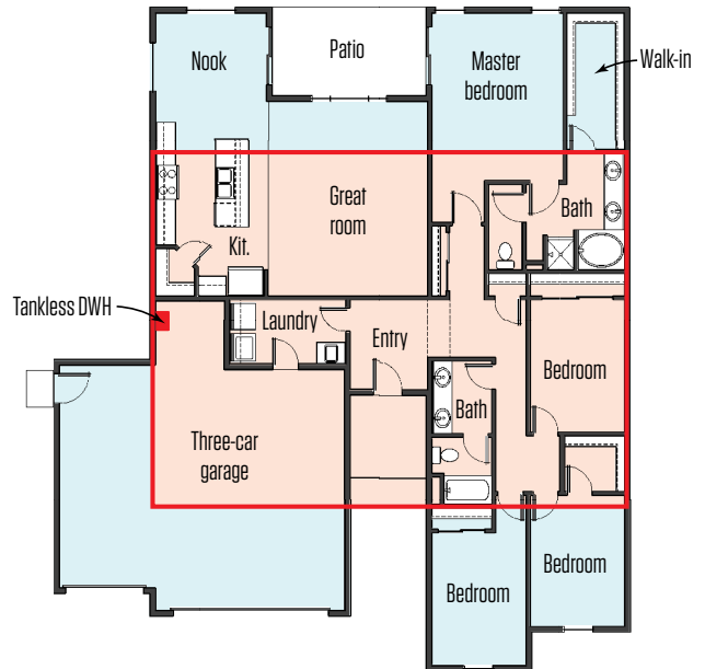
Hot Water System Rectangle ~81% (1,628 sq. ft.) of total square footage (2,010 sq. ft.)
