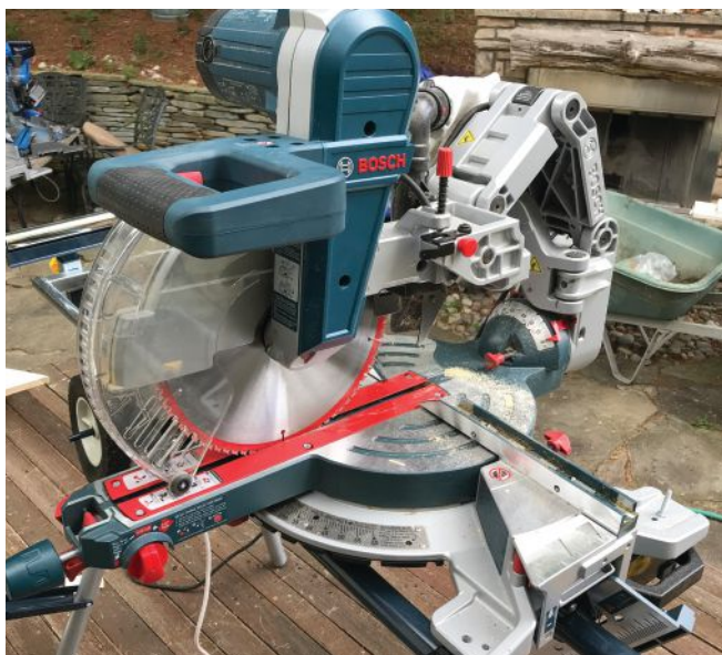
Accurate right out of the box, Bosch's GCM12SD has a beefy, well-designed fence system and efficient dust collection.
