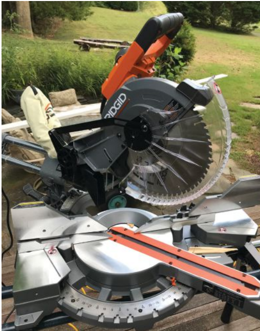
Ridgid's value-priced R4221 is capable of cutting 67-degree miters both to the right and to the left—best in class.
