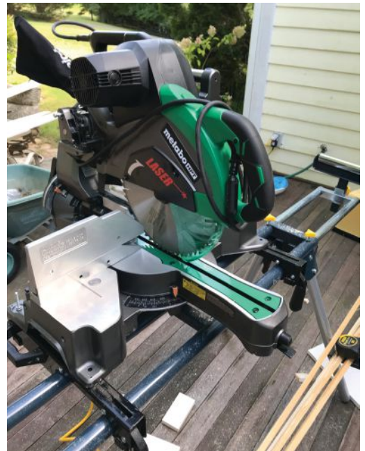
The least expensive saw in the group, Metabo HPT's C12RSH2 has a compact footprint and offers good dust collection.
