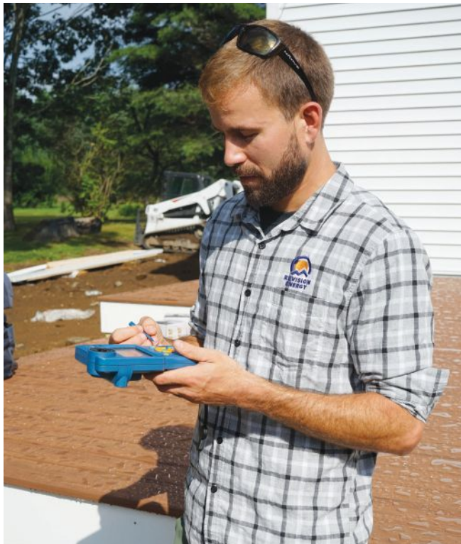
ReVision Energy's Thomas Tutor demonstrates use of the Solmetric SunEye for determining solar exposure.
