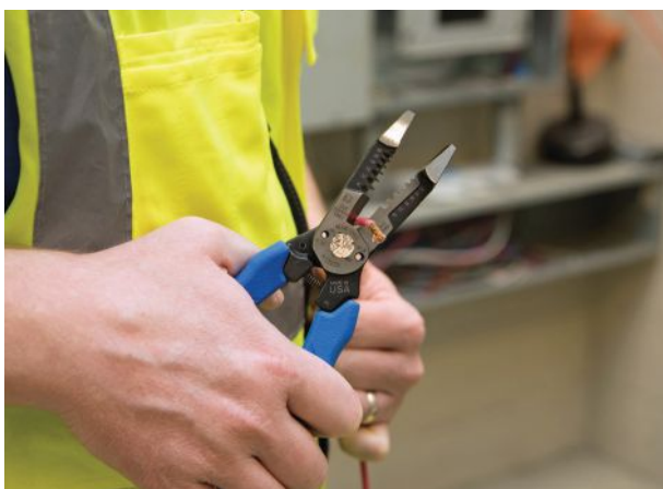
Klein-Kurve wire strippers have comfy handles, shear-cutting knives for cutting wire and cable, and a large, knurled plier head for pulling and twisting wire.
