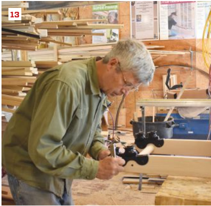
The author attaches the roller hardware to the tops of the ladder rails (13). After drilling holes, he installs the spreader rods, which are held at each end with cap nuts (14). The bottom roller hardware is the last part to attach to the ladder (15).
