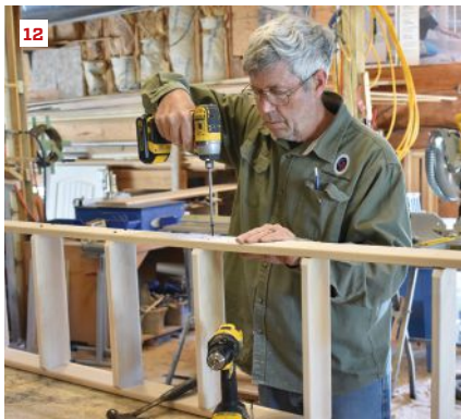
After predrilling for the screws, the author attaches one rail to the treads and the top rung (11). He then flips the assembly over and attaches the other rail (12).
