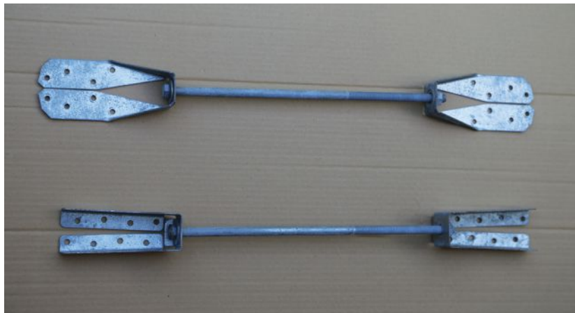
Figure 2. The two most common 1,500-lb. deck lateral-load ties are the Simpson Strong-Tie DTT2 (top) and the MiTek/USP DTB-TZ (bottom). Two are needed per connection, along with a 1/2-inch-diameter bolt or threaded rod, and structural screws to mount the hardware to the framing.
