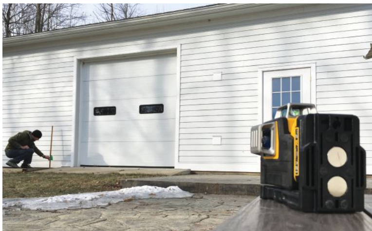
While the laser is mainly for indoor use, the beam, though faint, is visible from a distance for marking deck ledgers and other exterior layout.
