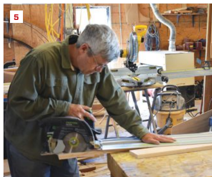
The author tacks two side rails together for milling (1). He spaces the treads (2) and draws layout lines with a rafter square (3). A stepped jig guides a router to cut the dados (4). He makes a cut at the top of each rail (5) and then rounds over the edges (6).
