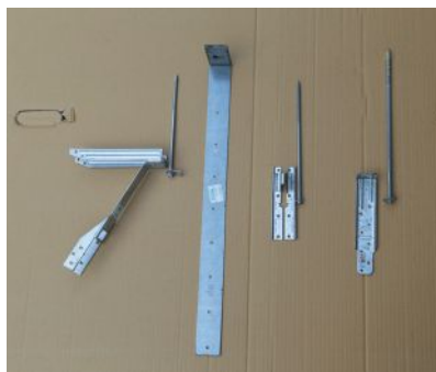
Figure 7. The IRC 4x750-lb. lateral-load detail is well suited for retrofits, since it doesn't require access to the house interior; here, an SST DTT1 tie connected to a \frac{3}{8} -inch lag screw embedded at least 3 inches into house framing is being fastened to the bottom of a deck joist (above left). Examples of hardware that meets the 750-lb. requirement include (above right, from left to right in photo) MiTek/USP ADTT, MiTek/LTS19, Simpson Strong-Tie DTT1, and FastenMaster LTS.
