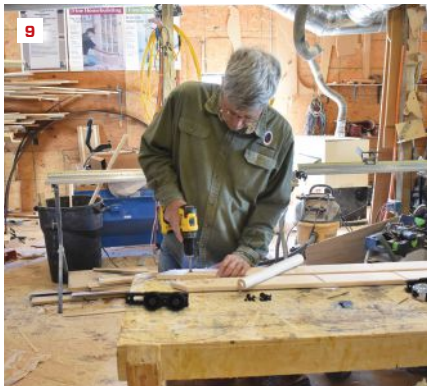
The author drills holes for the rollers (7) and a pilot hole for the top rung (8). He drills a slot for the top rung (9) and uses a jig for the tread attachment screws (10).
