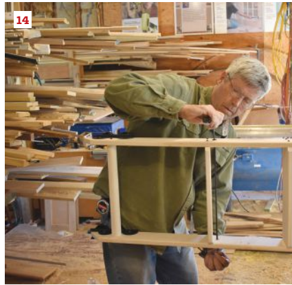
The author attaches the roller hardware to the tops of the ladder rails (13). After drilling holes, he installs the spreader rods, which are held at each end with cap nuts (14). The bottom roller hardware is the last part to attach to the ladder (15).
