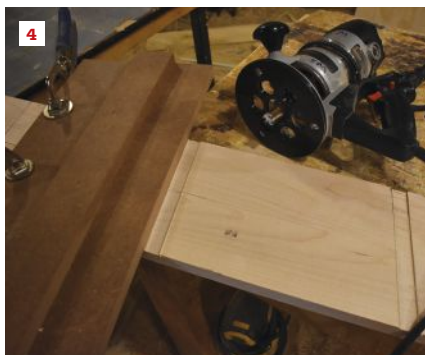
The author tacks two side rails together for milling (1). He spaces the treads (2) and draws layout lines with a rafter square (3). A stepped jig guides a router to cut the dados (4). He makes a cut at the top of each rail (5) and then rounds over the edges (6).
