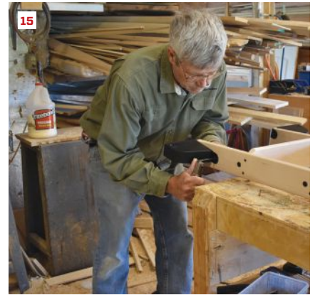
The author attaches the roller hardware to the tops of the ladder rails (13). After drilling holes, he installs the spreader rods, which are held at each end with cap nuts (14). The bottom roller hardware is the last part to attach to the ladder (15).
