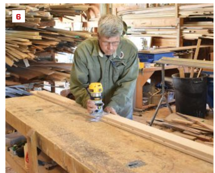
The author tacks two side rails together for milling (1). He spaces the treads (2) and draws layout lines with a rafter square (3). A stepped jig guides a router to cut the dados (4). He makes a cut at the top of each rail (5) and then rounds over the edges (6).
