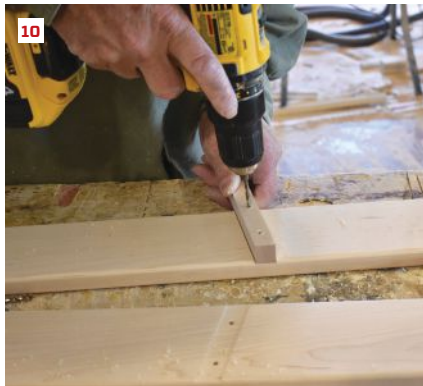
The author drills holes for the rollers (7) and a pilot hole for the top rung (8). He drills a slot for the top rung (9) and uses a jig for the tread attachment screws (10).
