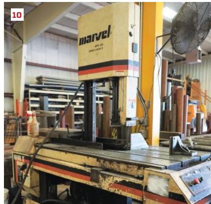
Cleanliness (7) and order (8) are signs of a well-run shop and a quality fabricator. Overhead cranes help move heavy beams safely around a shop (9). Tools typically found in a metal shop include beam saws (10) and punches called “ironworkers” (11).
