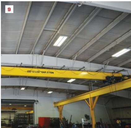
Cleanliness (7) and order (8) are signs of a well-run shop and a quality fabricator. Overhead cranes help move heavy beams safely around a shop (9). Tools typically found in a metal shop include beam saws (10) and punches called “ironworkers” (11).
