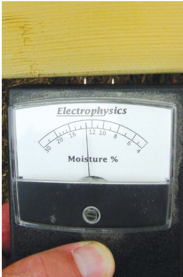
Figure 5. Measure, don't guess. A moisture meter should be used before applying any finish to make sure the moisture content throughout the decking is within an acceptable range, typically less than 15%.
