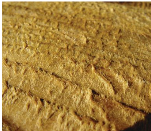
Figure 4. Pressure washing is effective at removing dirt and failing finishes (A). Be sure to match the tip size (B) to the operating pressure of the unit to avoid damage to the wood (C). After power washing, use a sander to remove the fuzzy wood fibers that have been raised during the process (D).
