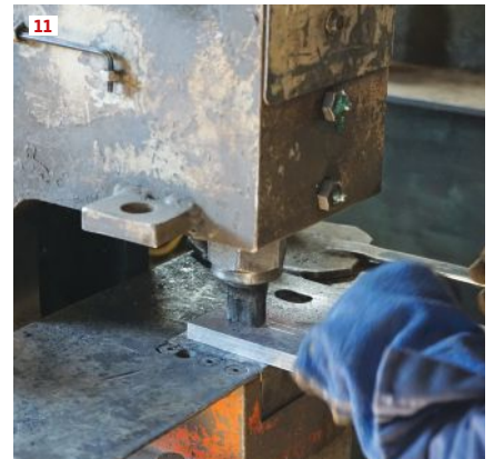
Cleanliness (7) and order (8) are signs of a well-run shop and a quality fabricator. Overhead cranes help move heavy beams safely around a shop (9). Tools typically found in a metal shop include beam saws (10) and punches called “ironworkers” (11).
