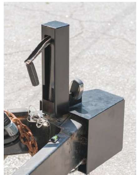
The Vault isolates the tongue and the crank (jackstand handle) from tampering and from the power tools or bolt cutters of would-be thieves.
