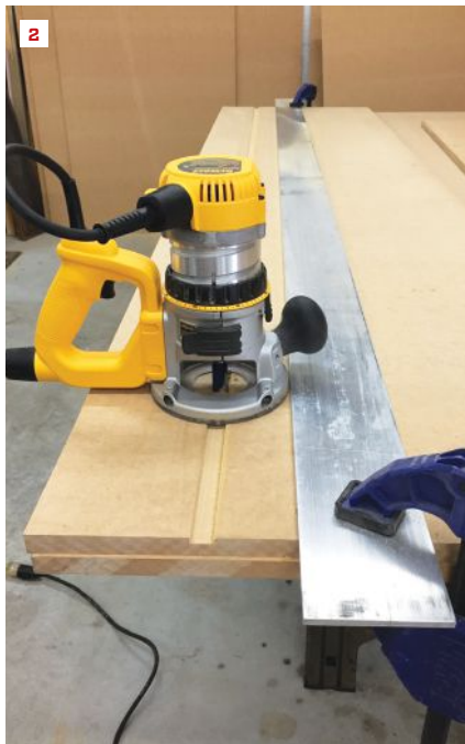
The author cut the toy-box parts from a sheet of 3/4-inch MDF, using an aluminum straightedge to guide the saw cuts (1). He used the same straightedge as a router guide for the long dado cuts (2). For shorter dados, he made an MDF guide, clamping the sides of the box together to make the dados identical (3). The box was then glued and pocket-screwed together (4).
