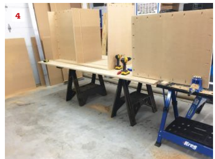
The author cut the toy-box parts from a sheet of 3/4-inch MDF, using an aluminum straightedge to guide the saw cuts (1). He used the same straightedge as a router guide for the long dado cuts (2). For shorter dados, he made an MDF guide, clamping the sides of the box together to make the dados identical (3). The box was then glued and pocket-screwed together (4).
