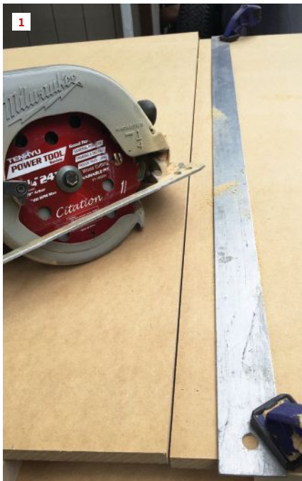
The author cut the toy-box parts from a sheet of 3/4-inch MDF, using an aluminum straightedge to guide the saw cuts (1). He used the same straightedge as a router guide for the long dado cuts (2). For shorter dados, he made an MDF guide, clamping the sides of the box together to make the dados identical (3). The box was then glued and pocket-screwed together (4).
