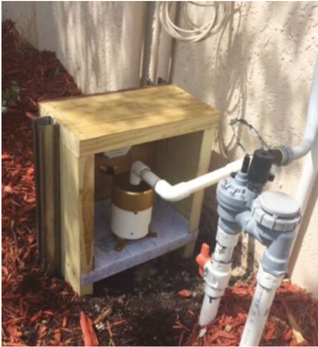
Lew Harriman and colleagues devised the system shown above to measure the water output of a house air conditioning and dehumidification system. Water emitted by the building's condensate drain filled a bucket, which tipped over when full (left); a pulse counter (right) counted the bucket tips, keeping a running total of the drain's performance.
