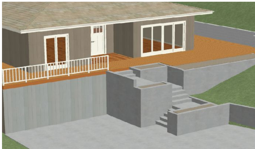
Figure 1. The existing deck had multiple problems, including a narrow staircase, poor illumination, multiple levels, and a non-code-compliant guardrail that blocked the view (photo, top). The author used a CAD program to flesh out the new design and provide accurate working plans for the concrete contractor (drawing, above).
