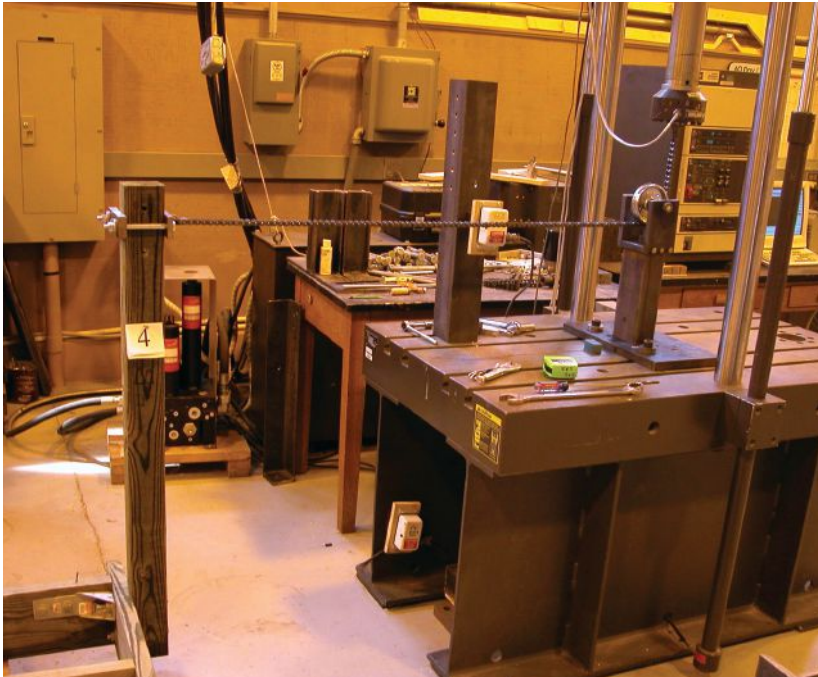
Virginia Tech researchers attached a chain to a guard post 37.5 inches (code requirement plus 1.5 inches) above the joists, over to a pulley, and up to a load cell. Raising the test machine load head produced a horizontal force on the post.
