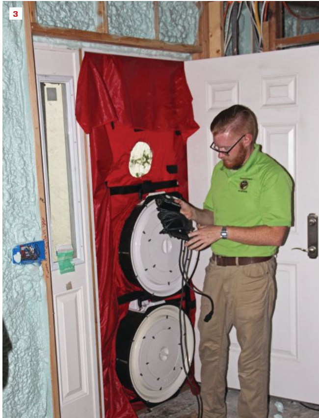
Technician Jack Hogan zeros the electronic manometer before the blower-door test (3). Hogan points out an air leak near the patio door (4). Hovis marks a gap in the foam insulation for correction by the foam crew (5).
