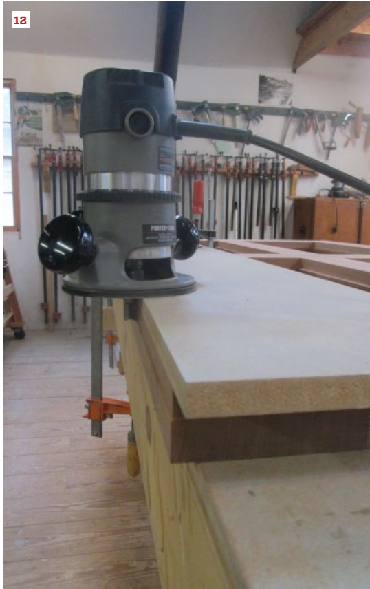
The door is too big to be cut to its finished size on a table saw. Instead, the author uses an MDF straightedge to guide a pattern bit to square the door to its final dimension (12). He then cuts the panels and prefinishes all the pieces with an initial coat of finish before installing the panels with an applied bead molding (13).
