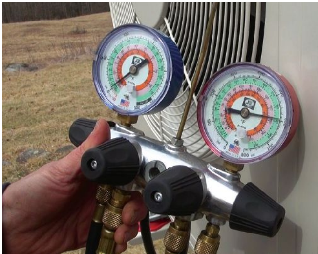
Technician David Ragsdale's pressure gauge shows the reading during a pressure test of the system at 600 psi (left) and during system evacuation at 170 microns (right) to purge moisture from the refrigerant lines.
