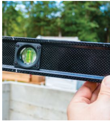
The DWHT43134 has two vials for plumb and one for level, two small hang holes, and small end caps that let you draw a line almost to the end of the level.
