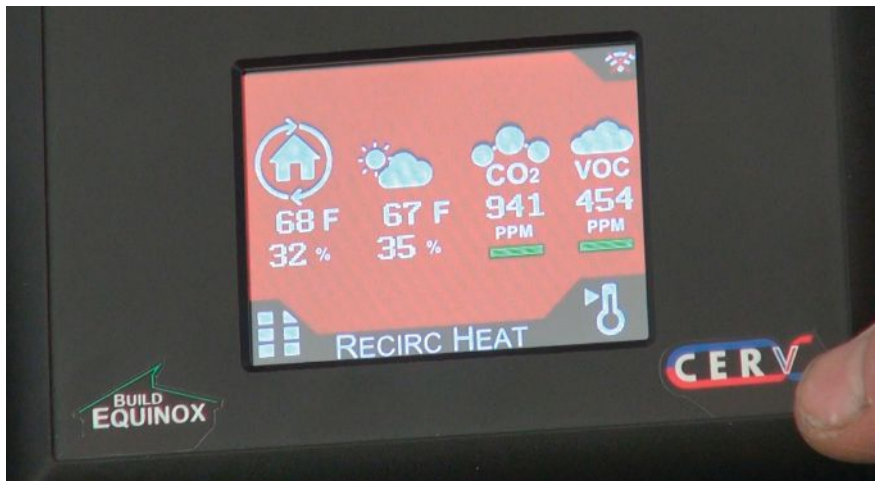
A close-up of the remote-control display for the Build Equinox shows readouts for temperature, humidity, carbon dioxide, and volatile organic compounds.
