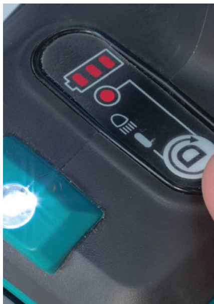
The screw gun has a handy fuel gauge. The “D” button turns the base-mounted LED light and the innovative “Push Drive” mode on or off.
