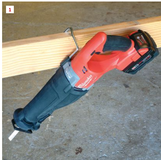
(1) The 2720 Sawzall includes a pivoting hook so you can hang it from framing, ladders, and scaffolding. (2) Thanks to its abundant power, long runtime, and cordless convenience, the M18 Fuel quickly became the author's go-to recip saw.
