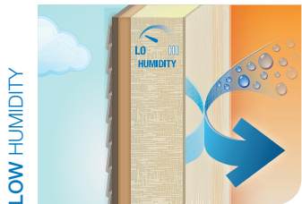
Remains moisture tight in winter when humidity in the cavity is low.
