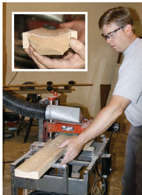
Figure 2. Spanish cedar boards were milled into fluted staves using a William and Hussey VFO6 molder. The custom-ordered knives, also from William and Hussey, cost around $150. It took one man one day to mill all the stock, making two passes per piece to avoid chattering while hogging out the ½-inch-deep cut for the fluted profile (inset).
